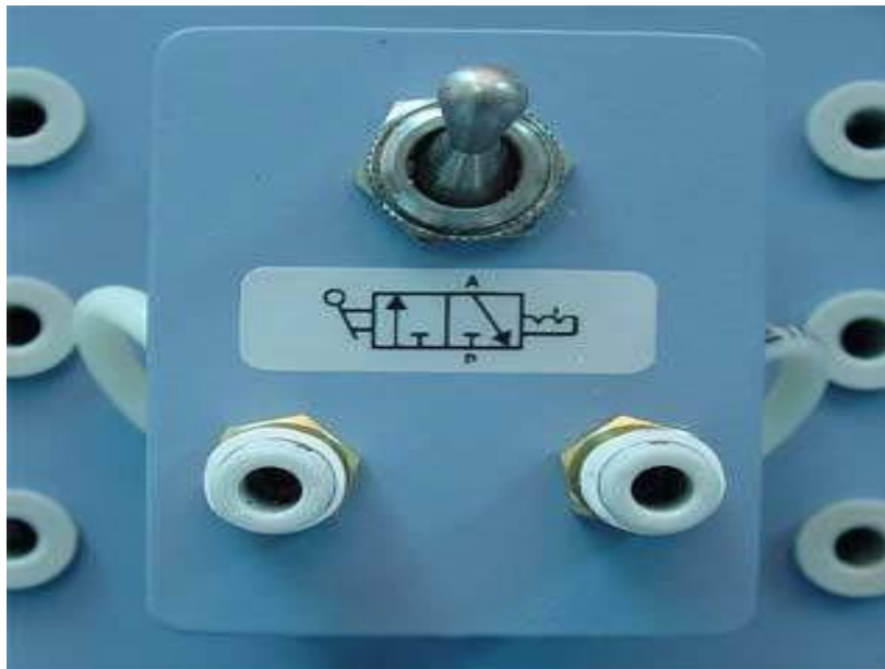
Fig. 10 (a) 3/2 directional control valve (b) Cross section
