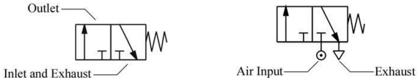
Fig 17 3/2 directional control valve (normally closed type)
